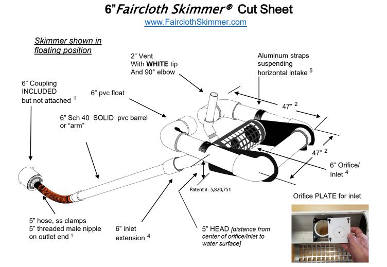
Hose can be attached to outlet using the threaded 5" nipple. Typical methods used: a) a metal structure with a steel stub out welded on the side at the bottom with a 5" threaded coupling or reducer(s);
