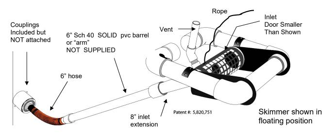
2. Glue the 6" sch 40 **barrel** at least 8' long to the 6" dark coupling on the **hose**.
