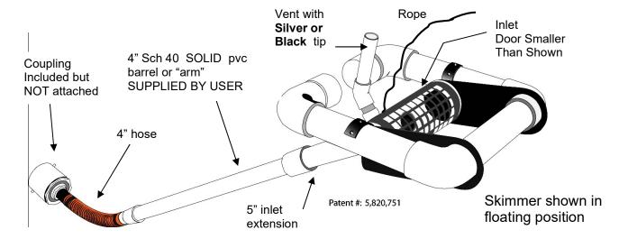
2. Glue the 8' long 4" sch 40 barrel to the 4" grey coupling on the hose.
