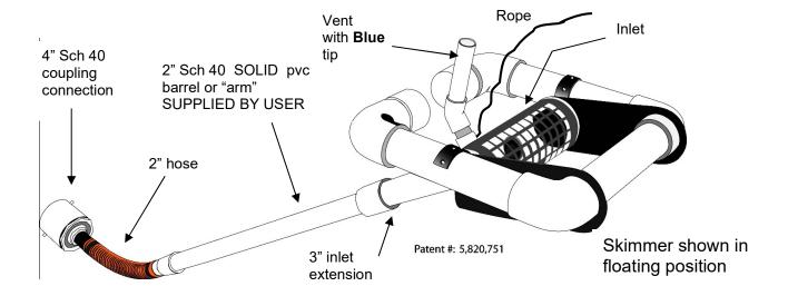
2. Glue the 8' long 2" sch 40 barrel to the 2" grey coupling on the hose.
