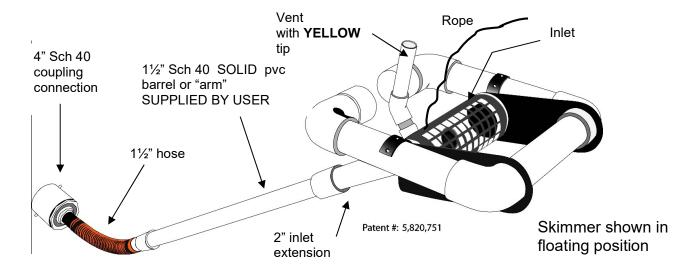
2. Glue the 6' long  $1\frac{1}{2}$ " sch 40 **barrel** to the  $1\frac{1}{2}$ " grey coupling on the **hose**.
