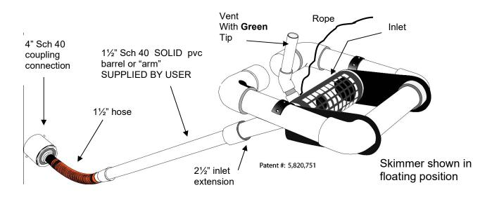
2. Glue the 6' long  $1\frac{1}{2}$ " sch 40 **barrel** to the  $1\frac{1}{2}$ " grey coupling on the **hose**.
